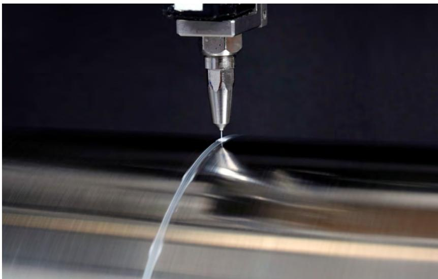
The new VINNAPAS® EP 6420 offers best-in-class performance for nozzle applications, showing excellent running stability without skin formation. This makes the VAE binder ideal for formulating water-based adhesives in demanding paper and packaging applications (photo: Wacker Chemie AG).
